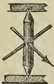
FIG. 1 The double pivoted needle of Petrus Peregrinus, A. D., 1269
